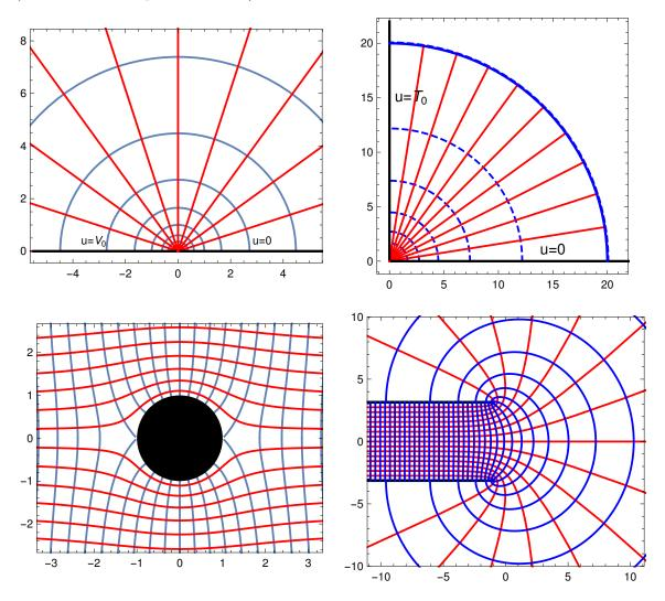
In the upper left we have the equipotentials (red) and field lines (blue, pointing clockwise) for the problem of two semi-infinite plates held at different potentials. It can also be interpreted as the velocity potential (blue) and streamlines (red) for water issuing from a narrow slit along the z-axis (in 2D, issuing from the origin).
