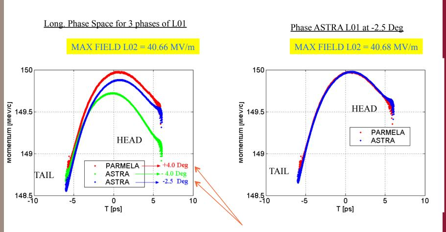
Note the reversal of the polarity needed here
