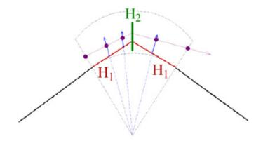
A drift-kick-drift in a bending magnet. Several kicks per element improve on the level of approximation with the real accelerator.
