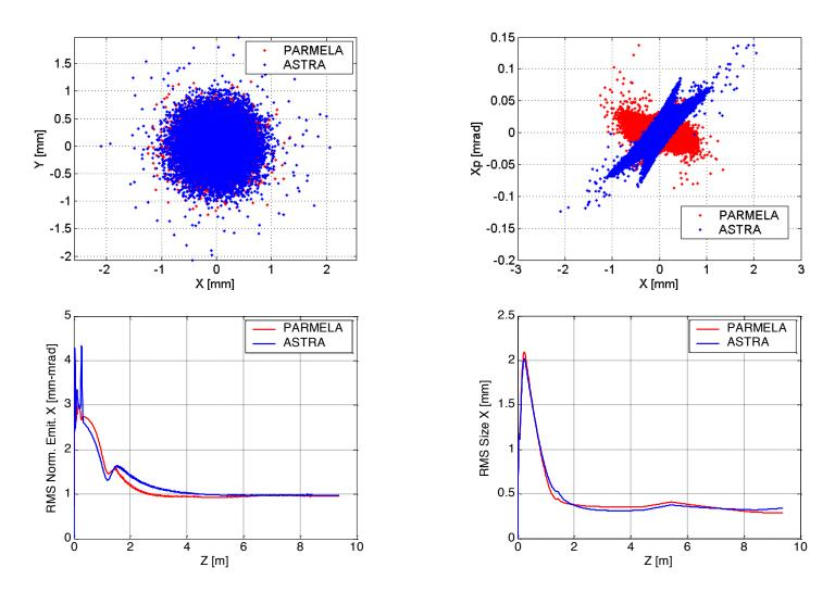
Agreement of transverse focusing is rather poor. Just looking at the Twiss functions derived from these data will be misleading.
